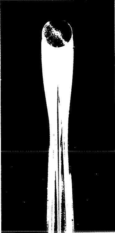
Figure 10: Snapshots of the near wake of a very small aspect ratio cylinder ( l/d=0.5 ). a) R=300 , b) R=450 , c) R=500 , d) R=750 , e) R=800 , f) R=900 .
