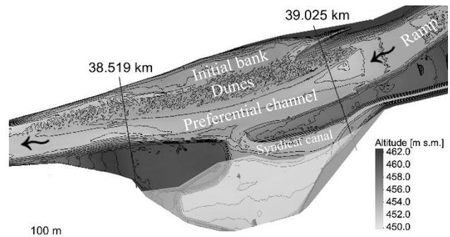
Figure 1: Bathymetry of the Verney widening at the end of the 100-year flood test (Lidar survey) and its configuration.
