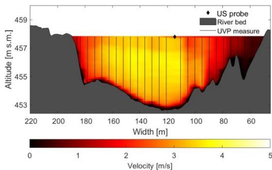
Figure 5: Velocity magnitude for the section km 39.025
