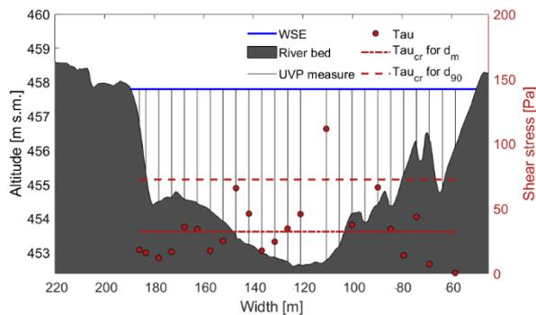
Figure 10: Shear stresses computed for the profile km 39.025
