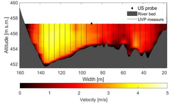
Figure 6: Velocity magnitude for the section km 38.519
