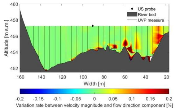
Figure 7: Variation rate between velocity magnitude and flow direction component
