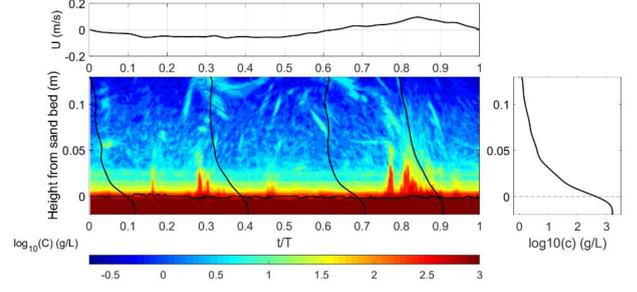
Figure 4: Free stream wave velocity (first line), intra wave mean concentration color plot (middle graph, in logarithmic scale) and mean wave-averaged concentration profile (right panel) for the low orbital velocity waves.
