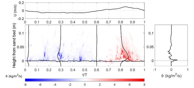
Figure 5: Free stream wave velocity (first line), intra wave mean flux color plot (middle graph) and mean wave-averaged flux profile (right panel) for the low orbital velocity waves.
