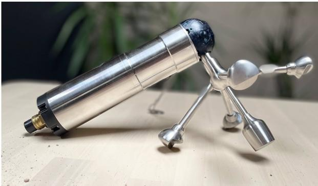
Figure 1: Mooring at low tide (top) and UB-Lab 3C (385 mm long with a central emitter and 4 surrounding receivers (bottom)
