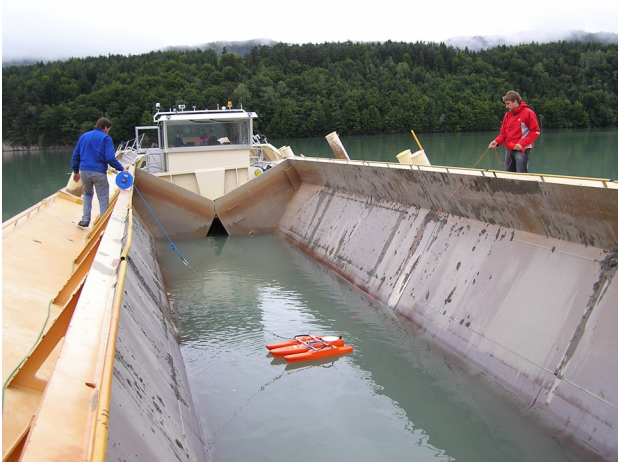
Figure 1: ADCP measurements with bottom-dump barge
