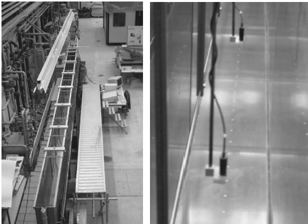
Figure 2: Photograph of the experimental flume (left) and the UVP transducer as well as the bottom and reference electrodes (right).
