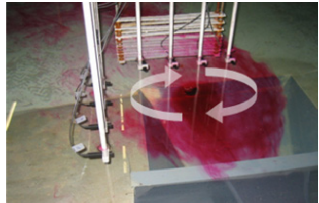
Figure 5: Measurement frame with 4x4 US transducers for vortices flow field mapping. A hydrogen bubble generator (in the back) was used for local hydrogen seeding supply.
